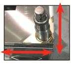
16. Using a 9/16" wrench, tighten-down the four bolts.
