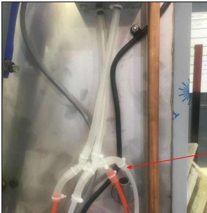
Back of machine showing use of existing mounting hardware for installation of vacuum switch assembly.
