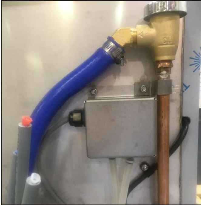
Back of machine showing use of existing mounting hardware for installation of vacuum switch assembly.
