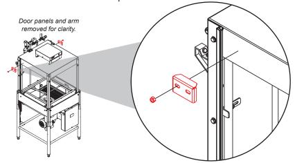
4. Secure top of panel to left side of hood using two slots on panel, then secure bottom to track assembly with hardware from Step 1.
