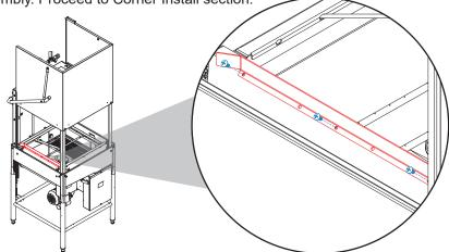
3. If using false panel, remove door stop bracket from wall side with 7/16 socket/nutdriver. Don't remove other door stop bracket.
