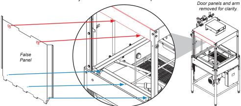
For right side against wall installation, remove drain handle before installing false panel.
